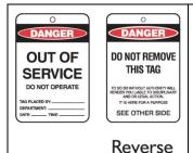
'Danger – Do not operate' Tag - A signed and dated label that is attached to energy isolation points of equipment, plant, pipes or lines by the person responsible for undertaking repairs, maintenance, service alteration or cleaning, to indicate isolation is in place and that plant, equipment, etc. shall not be operated. It shall only be removed by the person whose name is on the tag.
